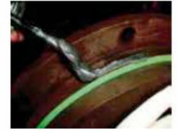
Smooth mixture of zinc dust and petrolatum grease that acts like an 'internal galvaniser' for superior protection of aluminum and ferrous surfaces from seizure and corrosion up to 400°C.
