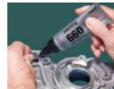
Used for repairing worn coaxial parts without re-machining. Enables reuse of worn bearing seats, keys, splines, tapers, or for retaining shims.
