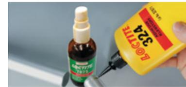
Activate reaction of Loctite®324 or Loctite® 325. No mixing required.
