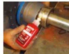
A controlled strength retaining compound, ideal for cylindrical parts that require disassembly; e.g. retention of bearings onto shafts and into housings.
