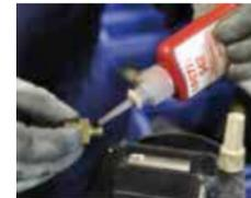
Recommended for threaded fittings as used in hydraulic and pneumatic installations.
